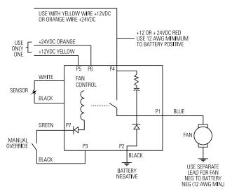
NOTE: This switch should be fused to prevent damage if ground is lost. A 30 amp fuse is required in the power supply.
